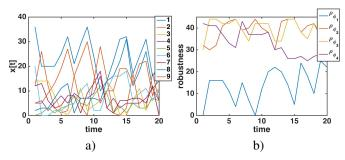
Fig. 2. a) The number of vehicles on each link b) robustness  $\rho$  measures the distance to the safety set boundaries. Notice that robustness is always above zero since the trajecory is always in the safe set.
