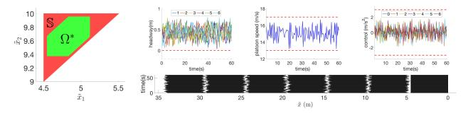
Fig. 2. Example 1: [left] Projection of the safe set  $\mathbb S$  and the RCI set  $\Omega$  on  $\tilde x_1$ - $\tilde x_2$  space. [right] Simulation of platoon of N=6. [Top, left to right]: Trajectories of headway, platoon speed and controls versus time [Bottom] Vehicular displacements in the leader frame.
