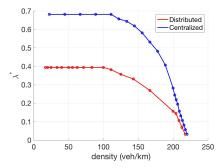
Fig. 5. Example 2: Density vs the magnitude of disturbances that the platoon can accommodate for centralized and distributed control architecture.
